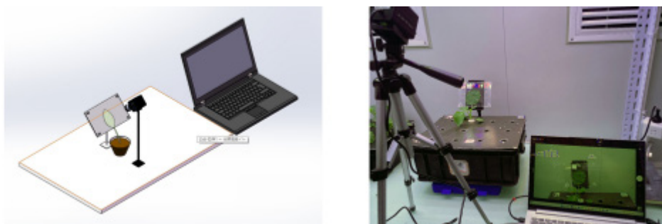
Fig. 3. Image-processing procedures for leaf-area measurement
