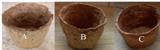
Fig. 1: Paper containers made from three biomaterials (A – Corn husk pot; B – Bamboo culm sheath pot; C – Banana pseudostem pot)
